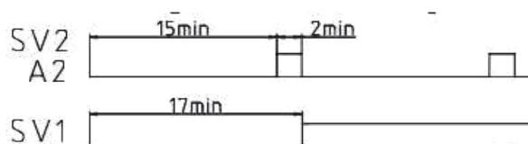
Figure 3, when the level is down to low position, lifting valve SV2 close 15min, open 2min
